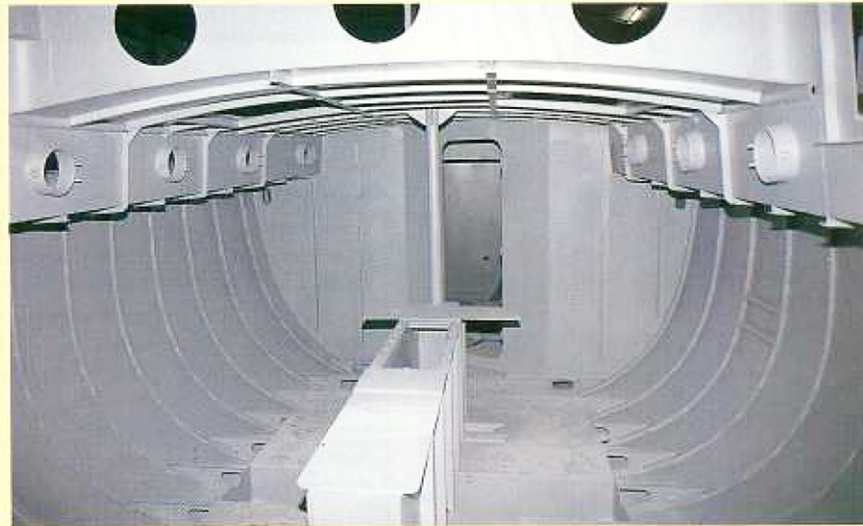
Above: the shot-blasted hull has been coated with a special primer. Left: swing keel mechanism before installation. Below: a bulky hull belies an impressive sailing performance
