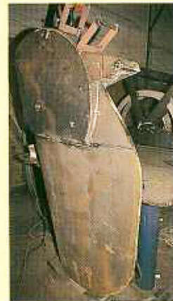
Above: the shot-blasted hull has been coated with a special primer. Left: swing keel mechanism before installation. Below: a bulky hull belies an impressive sailing performance
